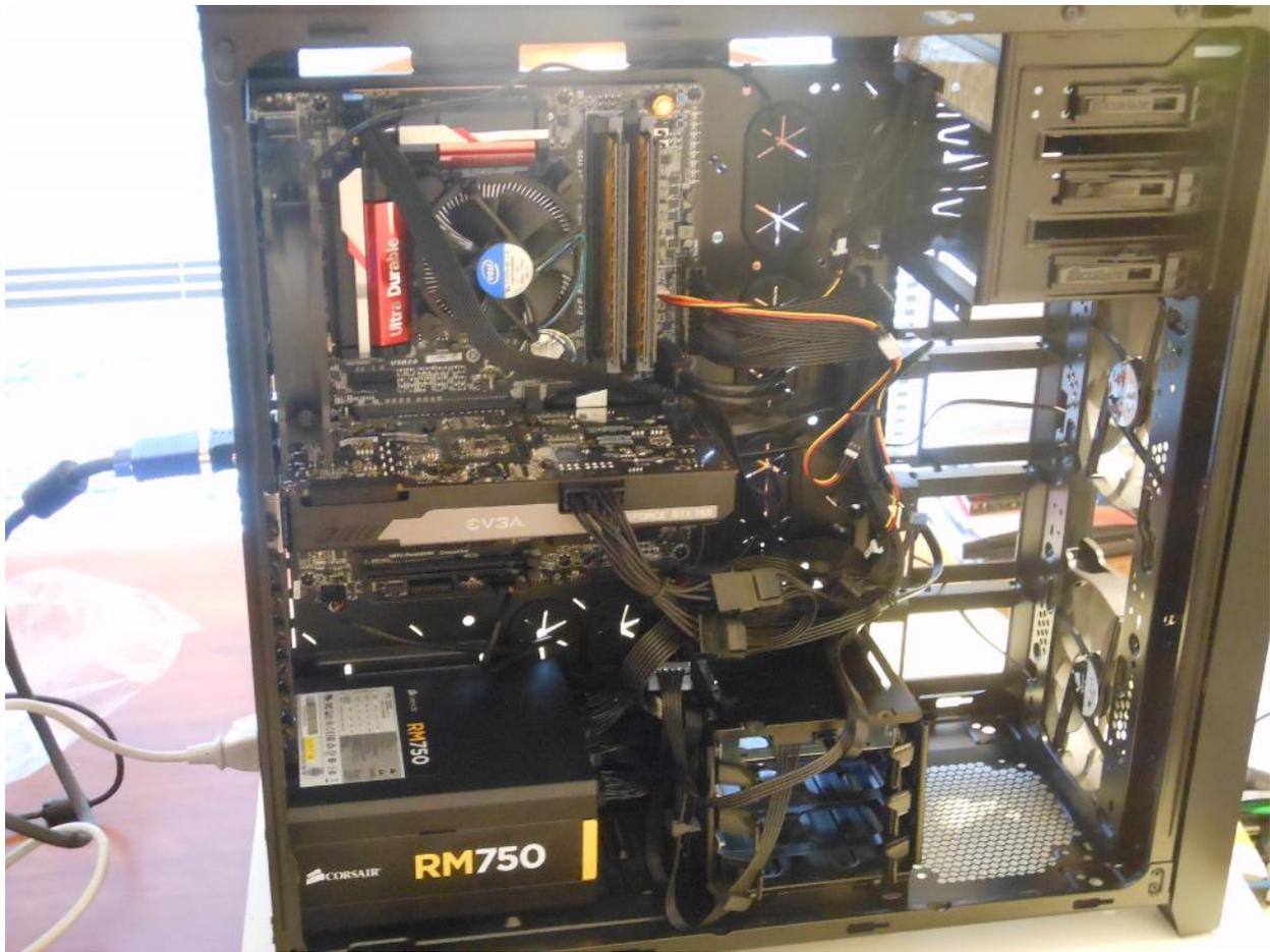
Took out one of the 2 hard drive cases to improve air flow. The case is capable of holding 8 drives, the most I'll put in will be 4, probably not even that many. The drives are "screw-less", you just slide them into the slot until they lock, same with the external drives.
