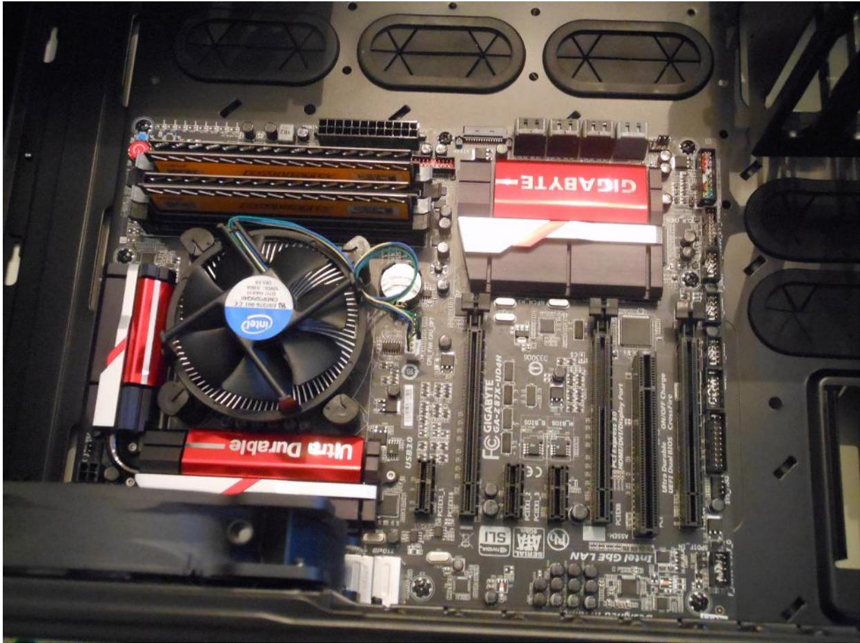
The motherboard after installing the RAM, microprocessor and heat sink. Very easy install, it just dropped into place, no modifications or extra hardware required.
