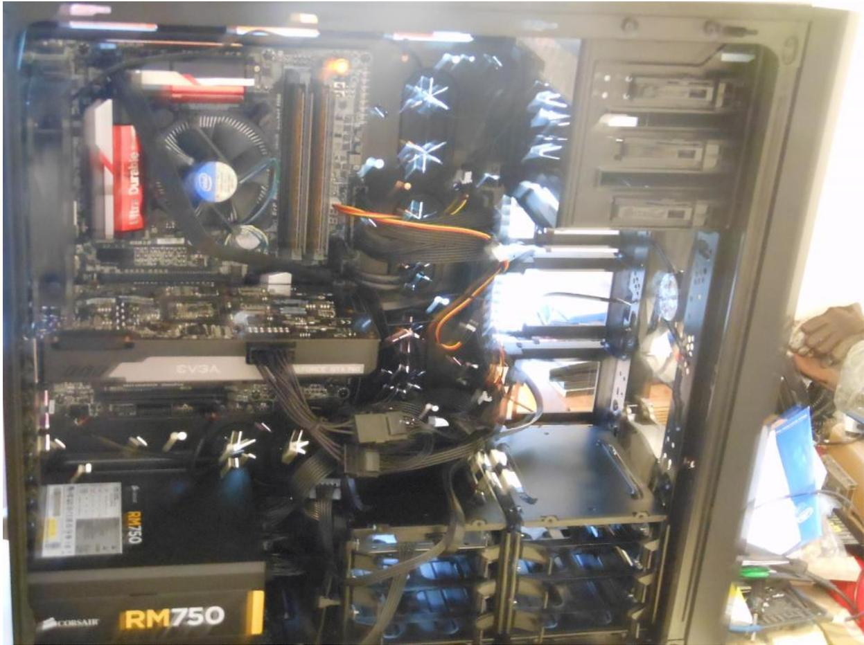
Had to add a splitter to the system fan jumper on the motherboard. My system has 3 fans currently—none of them have speed control. The motherboard has jumpers for 4 fans, including the system fan jumper, but 3 of them are speed control—4 pins instead of 3. So I had to get either an adapter, or a splitter. Building one if I had the parts to do it would have been an option too, but the cables are so cheap it's not worth the time to build your own cable.
